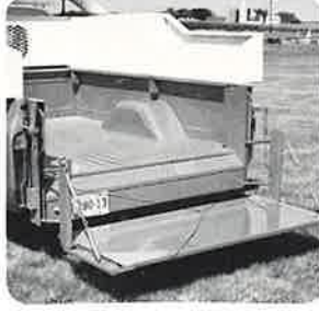
(4) The 900 lb. capacity electric hydra-load gate fits any standard pickup. The completely enclosed mechanism is operated with only one control lever and requires only one wire to the battery for operation. The big 28" platform can be used as a regular drop tail gate and it doesn't fold above the box when closed.
