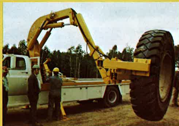
Tri-axial movement of Tirehand 10 enables precision placement of tire.
