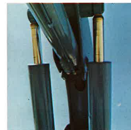
Shown here beneath secondary cylinder is a positive locking safety valve. An added safety feature on all hydraulic cylinders.
