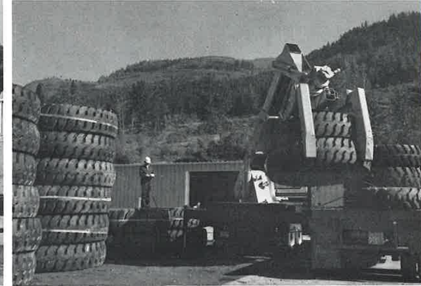
Handling two tires at a time, storage and stacking of the largest tires in the world is done quickly and efficiently.
