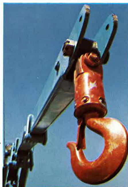
Hydraulically telescoping boom extends a full 40" beyond secondary boom.
