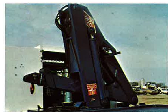
LEFT: Figure "4" Shaped traveling position takes only 28" of deck space.
