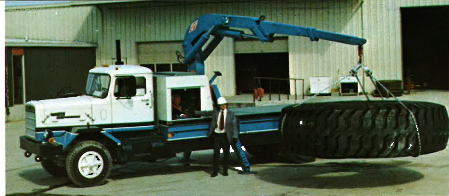
Horizontal or vertical positioning of the 40.00 x 57 tire is easily accomplished with the Mantis 10,000 and the giant sling.
