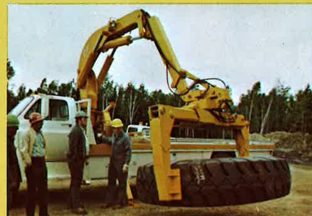
Grasping tire in a vice-like clamp, the operator completes tire change without leaving crane controls.
