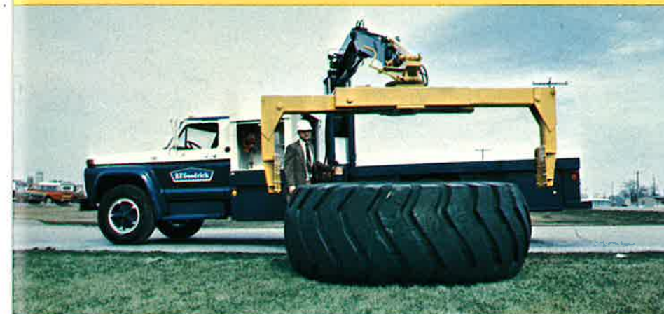
Hydraulically telescoping arms extend 107" to handle large tires.
