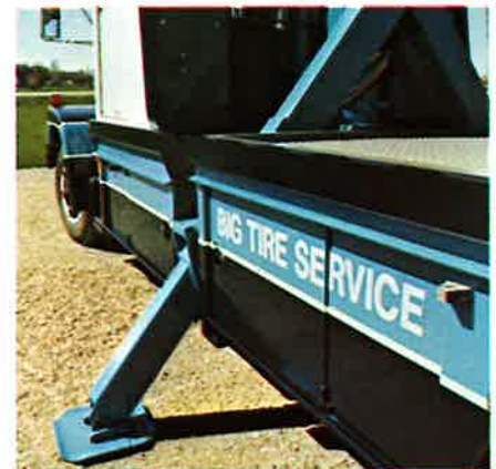
Two-piece split body construction allows free movement of lateral outriggers.
