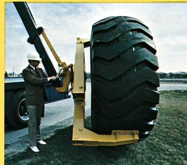
360° manual rotation of Tirehand 7 enables accurate and easy positioning of tire.
