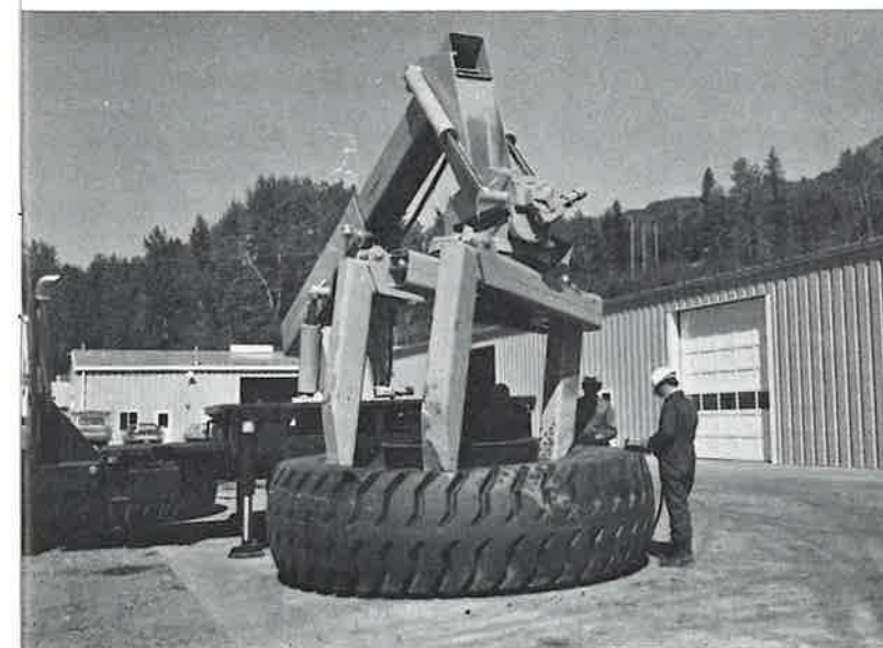
Rim removal is quickly accomplished with clamp in close quarter position.
