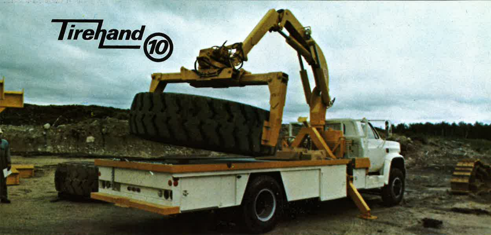
360° manual rotation of Tirehand 7 enables accurate and easy positioning of tire.
