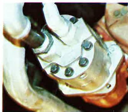
P.T.O. attached directly to hydraulic pump eliminates all drive lines.
