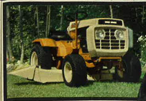
F 4-speed tractor with transaxle drive
